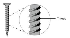
The finer the pitch of the screw, the more turns are required, but the less effort is needed to drive the screw in. The load is the friction and other forces exerted by the wood on the screw.
