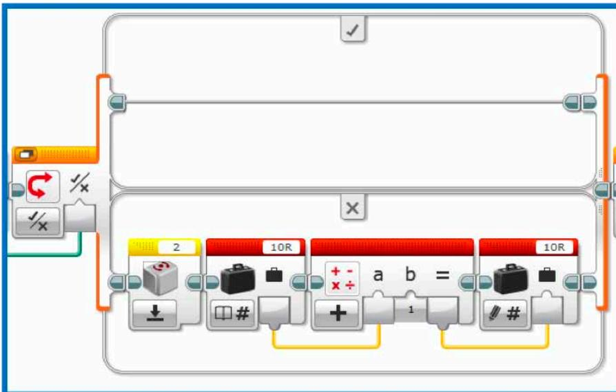
The operation executed in program part C depends on whether the number of rotations determined is greater or less than  $10$ . If the number of rotations is less than  $10$ , nothing happens. If the number of rotations is greater than or equal to  $10$ , reset the Gyro Sensor and increase variable  $10R$  by  $1$ .
