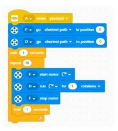
Have students test the program. What happens? The students must have a force sensor attached in order to start the program running by a press. The model does not have a force sensor attached; therefore, the program will not run. How can you fix the program? **Hint:** Choose a different start block.
