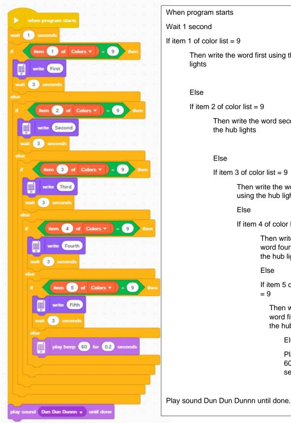
If item 1 of color list = 9Then write the word first using the hub If item 2 of color list = 9Then write the word second using the hub lights Else If item 3 of color list = 9 Then write the word third using the hub lights Else If item 4 of color list = 9Then write the word fourth using the hub lights Else If item 5 of color list = 9 Then write the word fifth using the hub lights Else Play beep 60 for .2 seconds
