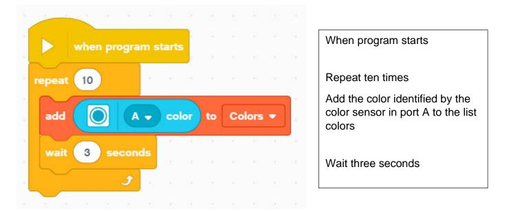
**Note:** When the program starts, the color sensor in Port A will read a color and add it to the list (array) named "Colors". It will wait three seconds and repeat reading and adding a color – 9 more times. The add block is new for students. It is located under Variables and is shown as add "thing" to Colors.
