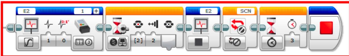
Starts the Brick Data Logging function for subsequent analysis on the computer. After pushing the EV3 Center Button, the Brick Data Logging function is ended, as is execution of the loop from program part C.
