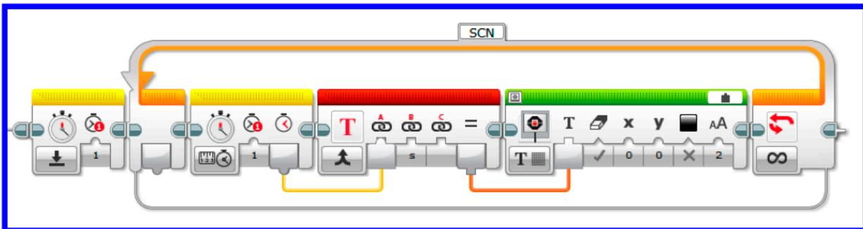
Commences at the same time as program part B. Resets the timer to 0 seconds, and then shows the elapsed time in seconds on the Brick Display. The loop is terminated in program part B.
