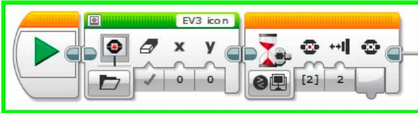
Shows the EV3 icon on the Brick Display, waits for the EV3 Button to be pressed.
