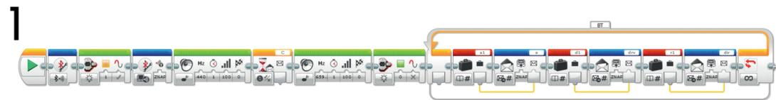
1 This first sequence sets up the Bluetooth connection. It first turns the connection on and uses the Brick Status Light in Yellow Mode along with sound to show the user what is happening. If and when the robots are connected, a Wait For Message Block is used to confirm the connection. Once that is activated, the Status Light is changed to green and another sound is played. The final loop, BTE, sends the messages from variables collected from other loops to the robot.
