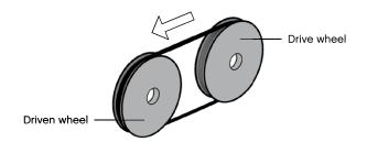
In a belt driven pulley a continuous belt joins two pulley wheels. The wheel to which an external force is applied (effort) is called the drive wheel, and the other the driven wheel. The drive pulley wheel provides the input force and the driven pulley wheel delivers the output force. When the drive wheel turns the belt moves and causes the driven wheel to turn in the same direction. If the drive wheel is smaller than the driven wheel, the driven wheel will turn more slowly than the drive wheel.
