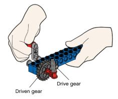
This model shows an idler gearing. The small gear is an idler gear. The idler gear does not affect the speed or output force of either the drive or the driven gears. The drive and the driven gears turn in the same direction and at the same speed.
