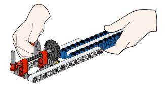
This model shows a rack and pinion gearing. Unlike the previous gears a rack and pinion gearing can only be used for linear motion, not rotary. When the handle is turned the gear rack moves forward or backwards depending on the rotational direction of the small gear (called a pinion).
