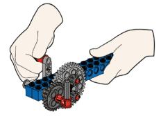
This model shows an angle gearing. The two meshed bevel gears transfer the speed and force unchanged, but at an angle of 90%
