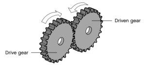
The drive gear is the gear that is turned by an outside effort, for instance your hand or an engine. Any gear that is turned by another gear is called a driven gear. The drive gear provides the input force and the driven gear delivers the output force.
