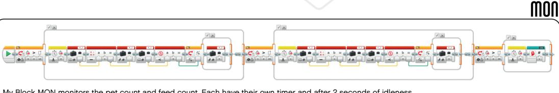
My Block MON monitors the pet count and feed count. Each have their own timer and after 2 seconds of idleness, the timers will reset and 1 is taken away from the count. An independent timer allows each count to run seperately when interacted with. Lastly, if there is no activity, timer 3 will run, and CS=1 will make the robot go to sleep.
