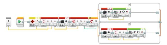
My Block MHT moves the head of the robot. By taking an input and subtracting that from the current position of the head, as read by the Motor Sensor Block, the motor is moved that amount of degrees at full power. The Compare Block and switch ensure the proper direction of movement.
