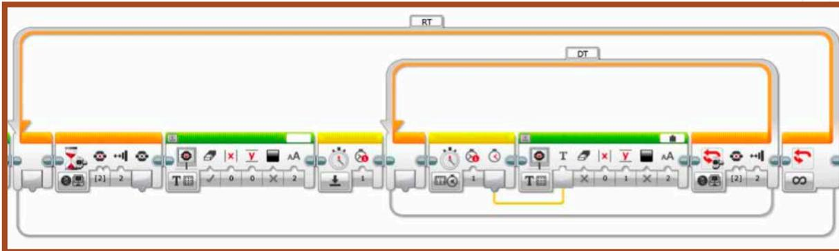
Program part A is a loop that executes repeatedly until the user exits the program by pressing the Cancel Button. At the start of the loop, the program waits until the user initiates time measurement by pressing the EV3 Center Button. After that, the EV3 Display is cleared and the timer is reset.
