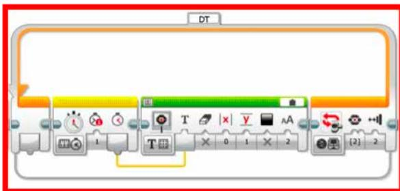
In program part B, the DT loop is repeated until the user ends it by pressing the EV3 Center Button. For each loop cycle, the time elapsed in seconds since the last timer reset from program part A is output on the Brick Display. If you end the loop, the last output time value in seconds remains on the display, and the program resumes at the start of program part A.
