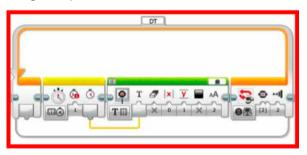
In program part B, the DT loop is repeated until the user ends it by pressing the EV3 Center Button. For each loop cycle, the time elapsed in seconds since the last timer reset from program part A is output on the Brick Display. If you end the loop, the last output time value in seconds remains on the display, and the program resumes at the start of program part A.
