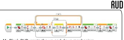
My Block RUD resets the up and down mechanism. The mechanism is moved up for .3 seconds, then loop UP begins. The switch checks to see if the motor current is reading anything other than zero. If it is, and the motor is still moving, the timer will reset. If it is no longer moving for 2 seconds, the loop ends. Lastly, the motor is moved back 20 degrees, and brake released at its starting position.
