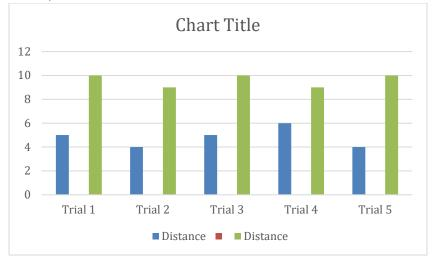
Distance with Brake On – Blue Distance with Brake Off - Green
